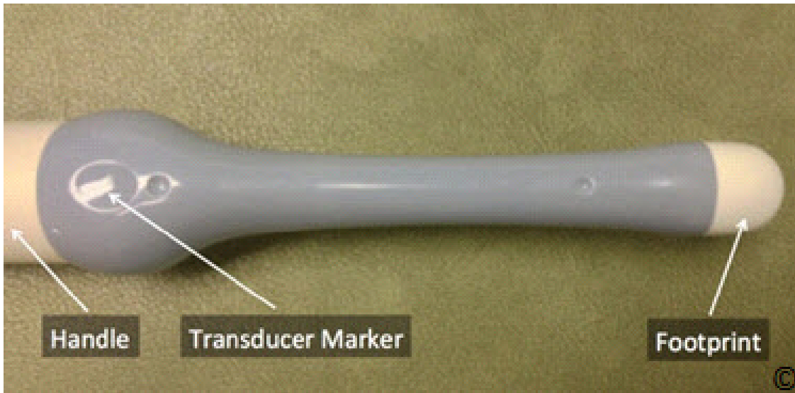
Figure 14.1: Transvaginal ultrasound transducer: note its shape like a long cylinder with a handle (labeled) and has a small footprint (labeled) at its tip that transmits and receives sound waves. The image also shows the transducer marker (labeled).
