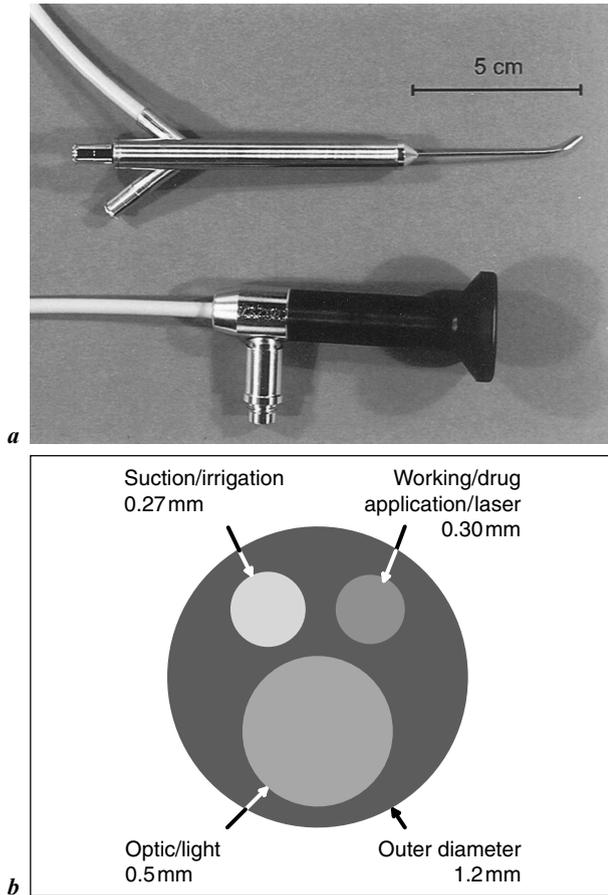
**Fig. 1.** Microendoscope developed in cooperation with Explorent GmbH/Stuemed GmbH® in particular for easy visualization of and drug delivery to the RW niche (*a*). It incorporates a thin fiber optic (6,000 pixels), a working/laser channel (0.3 mm i.d.) and an irrigation/suction channel (0.27 mm i.d.) allowing a total endoscope diameter as small as 1.2 mm. (*b*) Cross-sectional view.
