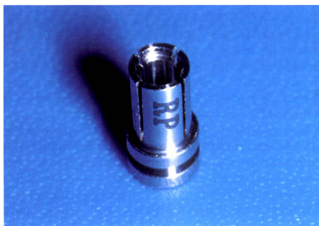
Fig. 10.14 Locating collar for use with a screw retrieval kit. This is placed over the top of the implant body to locate the rotating instruments used for removal of fractured screws.
