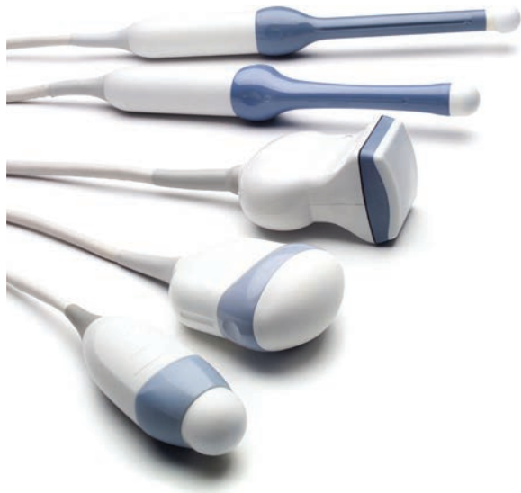
Figure 32-6 Mechanical 3D/4D transducers contain a motor within the transducer housing that provides a consistent automated sweep. Endocavitary, high-frequency linear, abdominal, and pediatric 3D/4D transducers are available. (Photograph courtesy of GE Healthcare, Wauwatosa, WI.)
