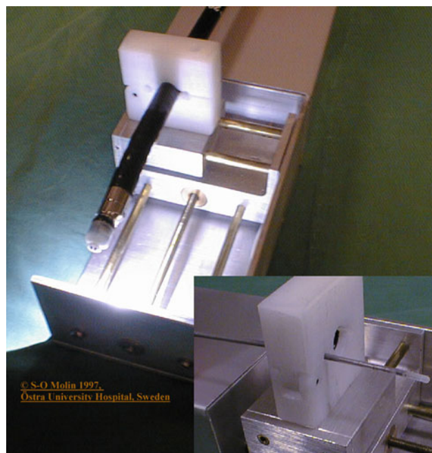
Fig. 10 A prototype acquisition unit for 3D EUS imaging that can be used both for echoendoscopes and miniprobes. The pullback system allows for a constant speed of transducer movement
