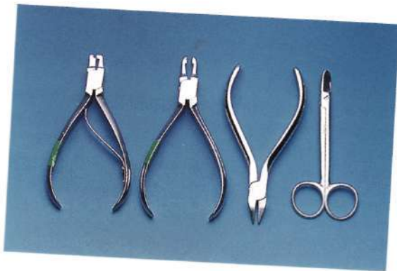
Figure 5.11 Pliers (Johnson 114) and crimping pliers (Unitek 800-108) are needed, although in our experience Adams pliers, readily available in most practices are adequate for crimping the crown margins. Crown cutting scissors, again available in most practices, are seldom required.
