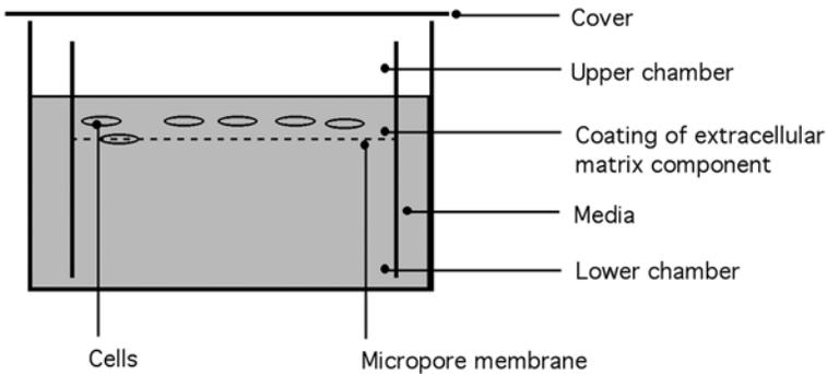
Fig. 1. Modified Boyden chamber system for the in vitro determination of cell invasion.
