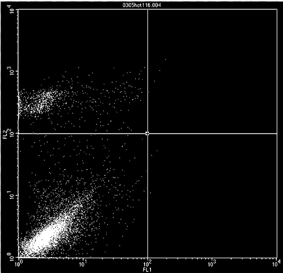
Fig. 5. Example of a profile in which a reagent is missing. In this example annexin-FITC has been omitted. The resulting appearance is equivalent to the PI-only control.
