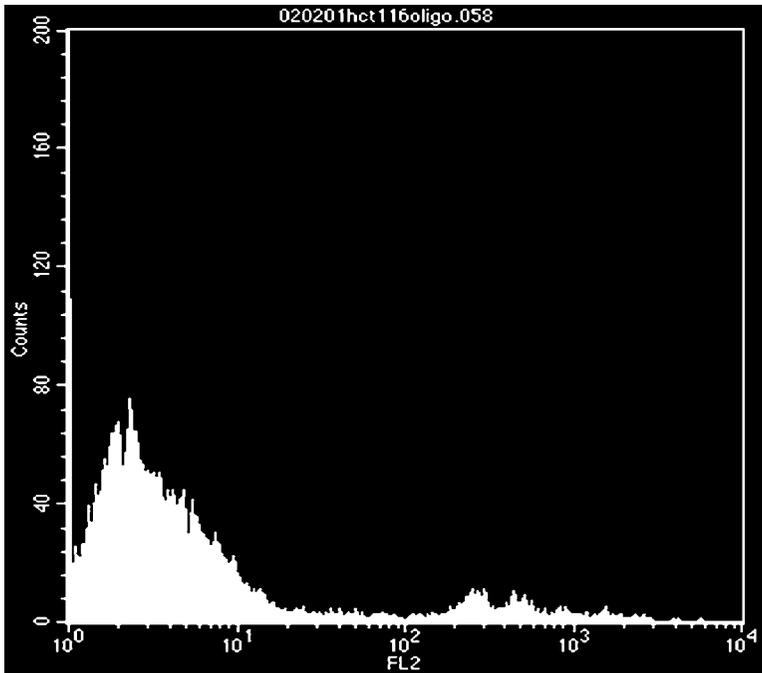
Fig. 8. Histogram of the red fluorescence from Fig. 7. Note the two peaks in the third decade corresponding to  $G_0$  and  $G_2$  peaks of the DNA histogram.
